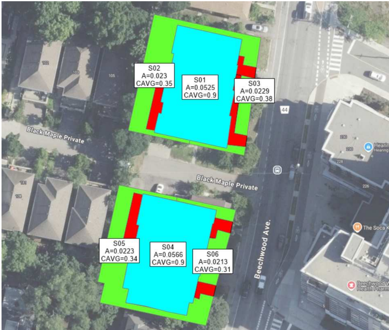
Figure 7-1 – Post-Development Storm Drainage
