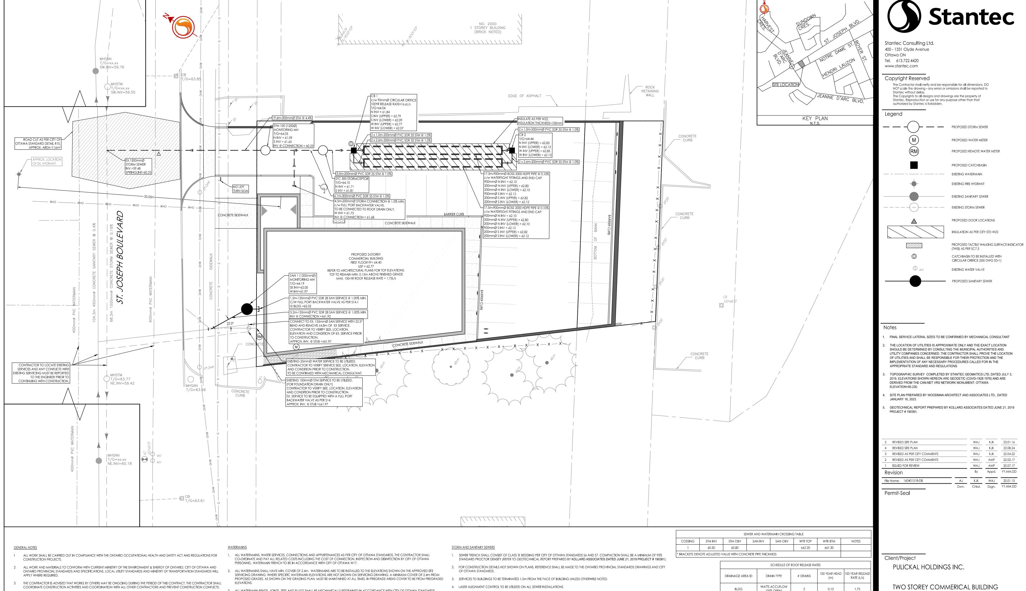
5. FROST PROTECTION PER CITY OF OTTAWA STANDARD DRAWING W22 WHERE THERE IS LESS THAN 1.8m OF COVER ABOVE THE SEWER SERVICES.
