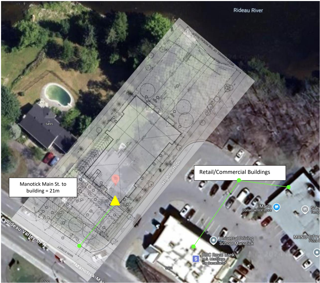
Figure 2.2 – Surrounding area 5497 Manotick Main St. with locations and distances of relevant noise sources with approximate site plan overlay.
