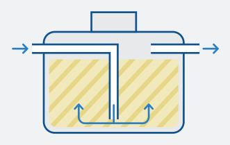
Water goes down to the bottom of the tank, then flows up through the media and out the outlet.
