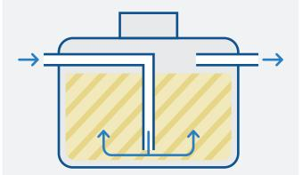
Water goes down to the bottom of the tank, then flows up through the media and out the outlet.
