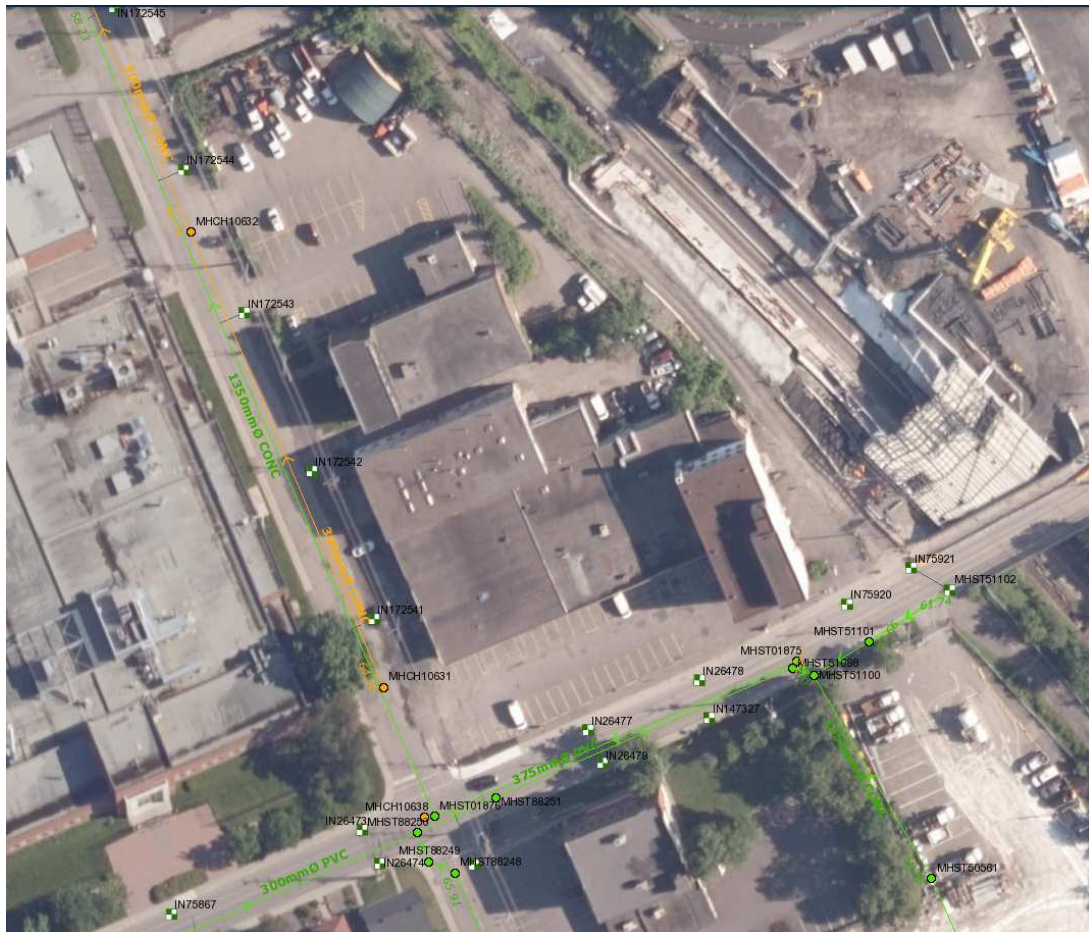
Figure 4-1 Existing Storm Sewer Services
