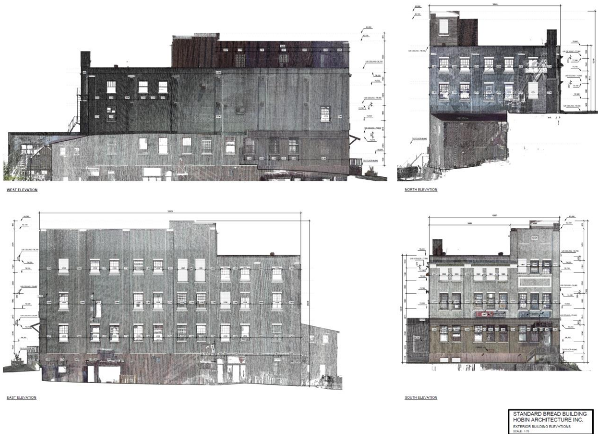
Figure 27: Photogrammetric recording of the Standard Bread Building. Source Hobin Architects
