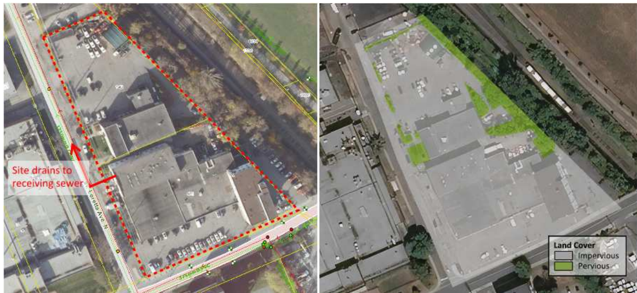
Figure 2: Existing Drainage (left) and Land Cover (right)
