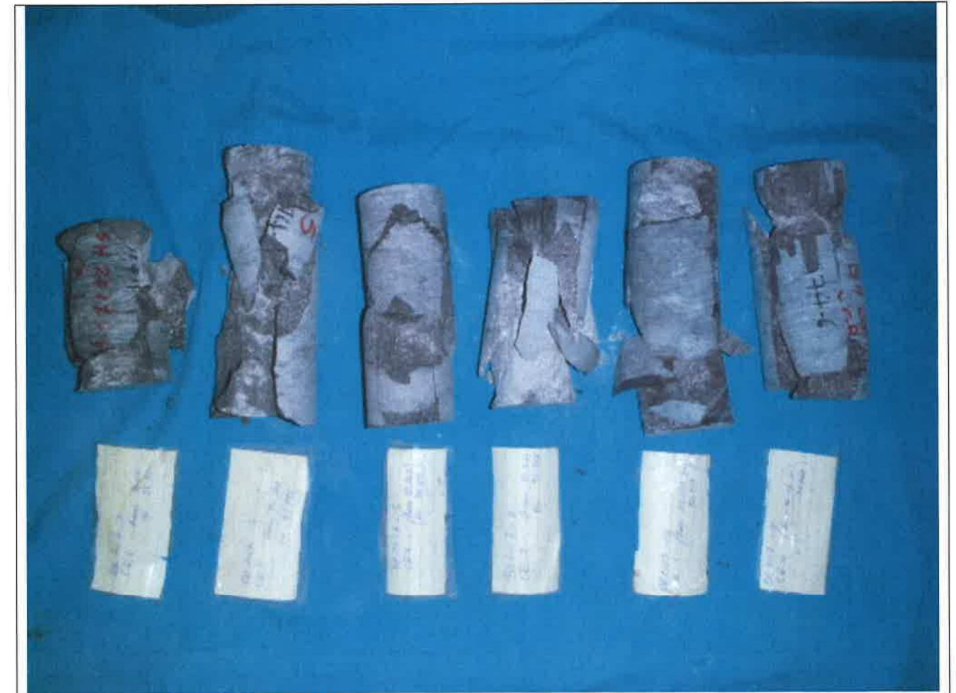
Photograph No. 1, Davroc Sample C974 -1 to 6, break failure after testing.
