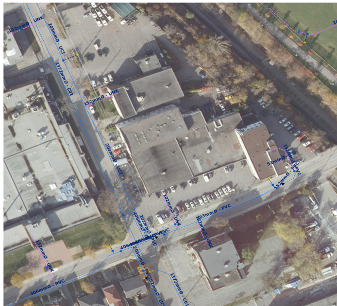
Figure 2-1 Existing Water Supply Services
