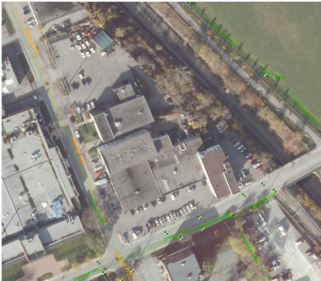
Figure 4-1 Existing Storm Sewer Services
