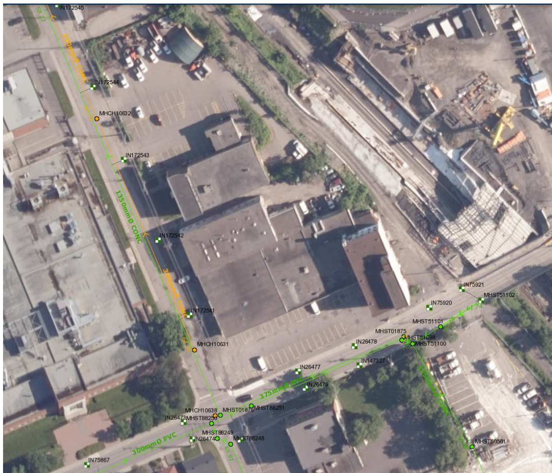
Figure 4-1 Existing Storm Sewer Services
