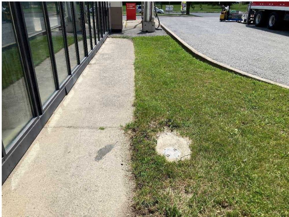
Photo 10: View of a monitoring well installed in a landscaped area west of the car wash
