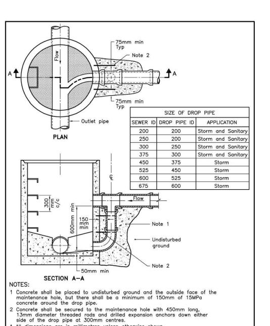
A All dimensions are in millimetres unless otherwise shown ONTARIO PROVINCIAL STANDARD DRAWING Nov 2016 Rev 3 CAST-IN-PLACE MAINTENANCE HOLE DROP STRUCTURE TEE OPSD 1003.010
