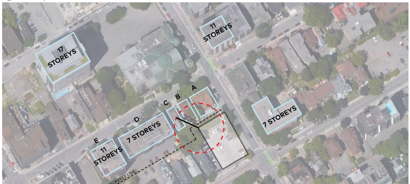
Figure 13 Building separation distance demonstration plan.
