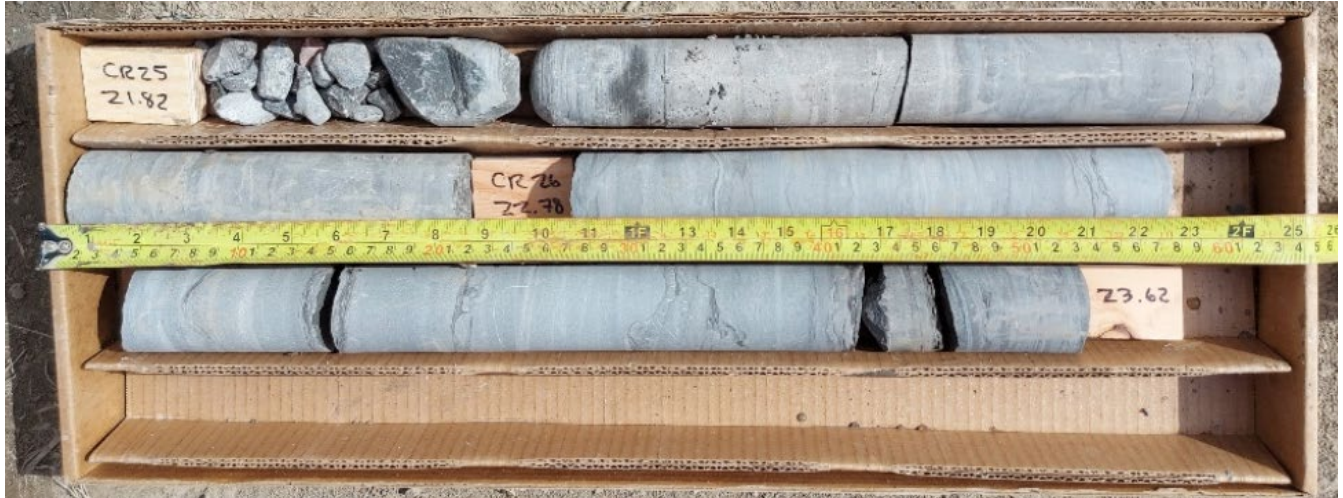
Photo 1 : BH-02 Core box – Dry rock
