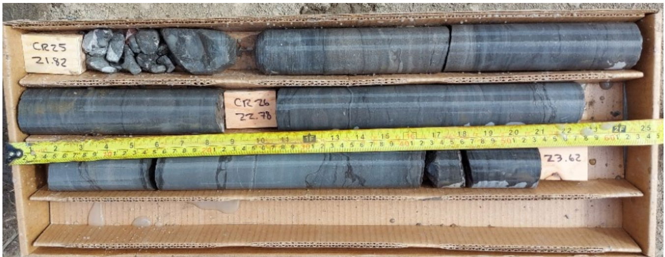
Photo 2 : BH-02 Core box – Wet rock
