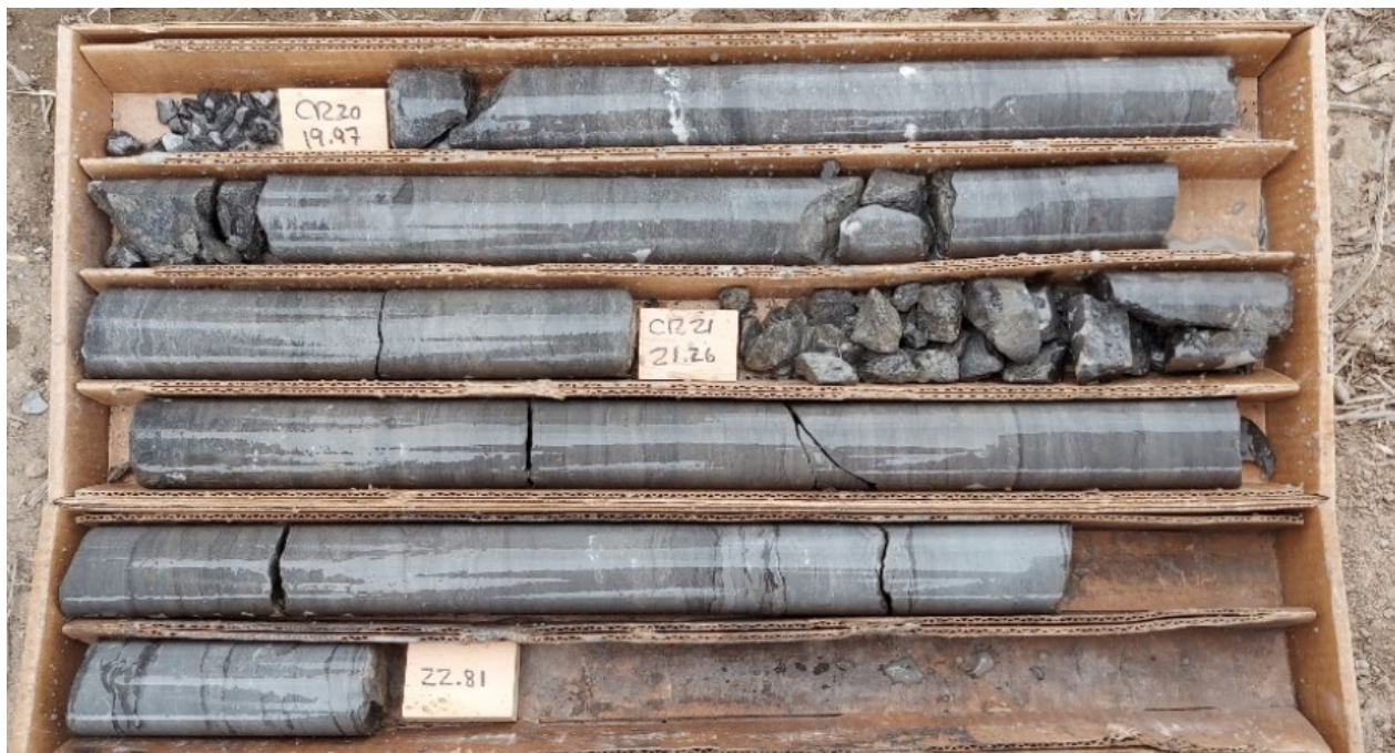
Photo 4 : BH-03 Core box – Wet rock
