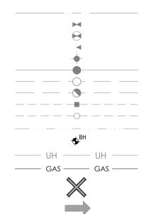
EXISTING WATERMAIN EXISTING VALVE AND VALVE BOX EXISTING VALVE CHAMBER EXISTING REDUCER EXISTING FIRE HYDRANT EXISTING SANITARY SEWER **EXISTING STORM SEWER** EXISTING CATCHBASIN MANHOLE **EXISTING CATCHBASIN** EXISTING SUBDRAIN CATCHBASIN EXISTING SWALE EXISTING BOREHOLE LOCATION EXISTING UNDERGROUND HYDRO EXISTING UNDERGROUND GAS
