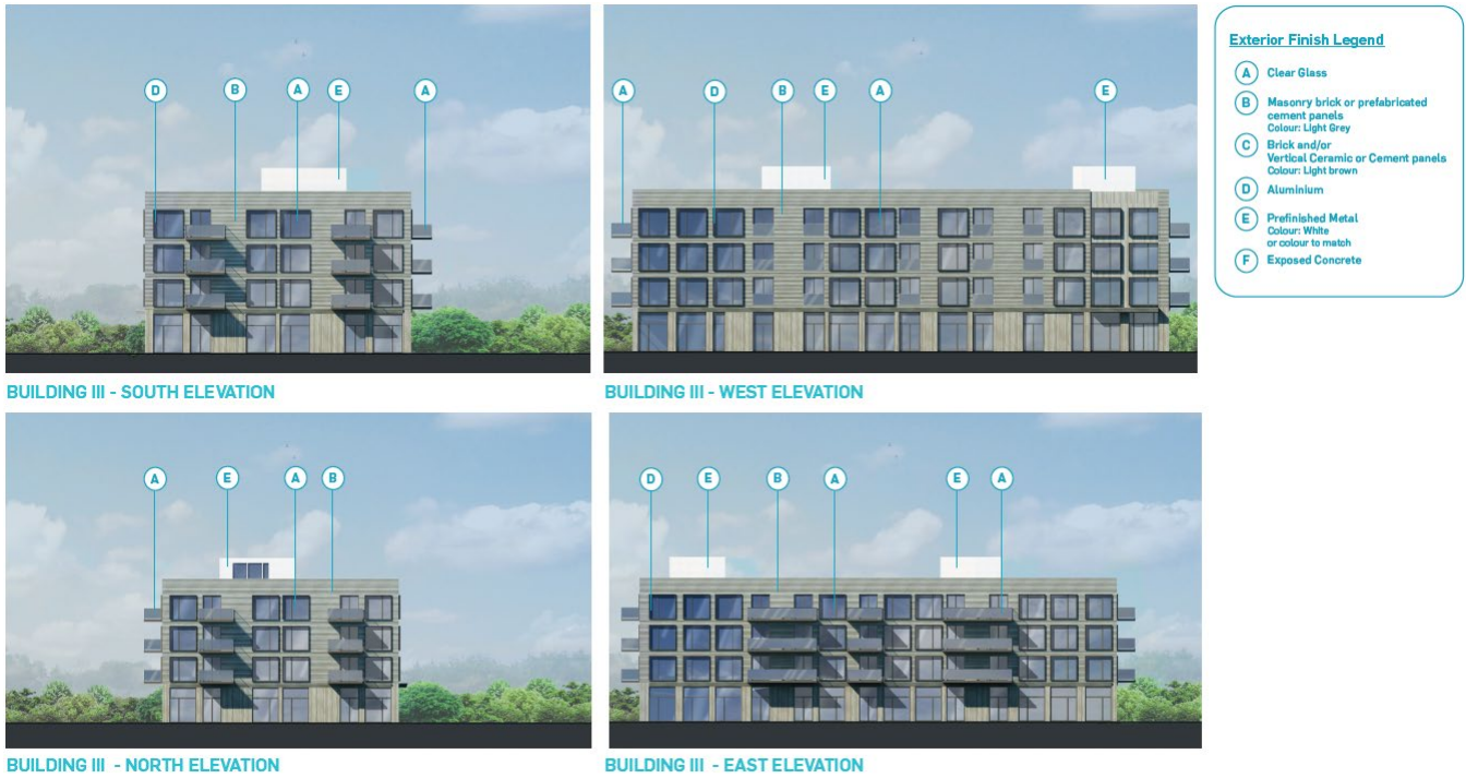
Figure 32. Building III design details.
