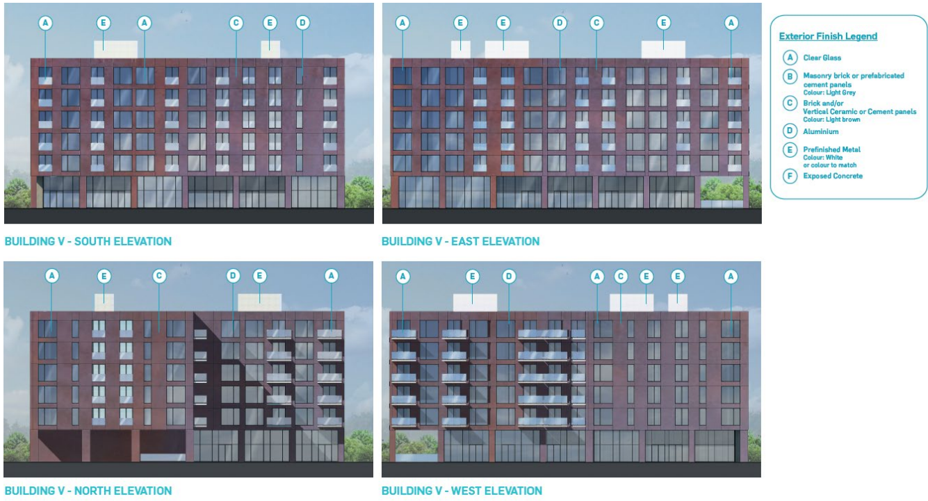
Figure 34. Building V design details.
