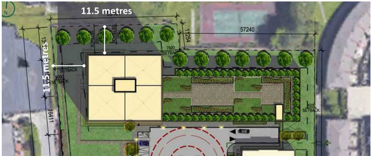
Figure 8: Tower Setbacks from Adjacent Properties.
