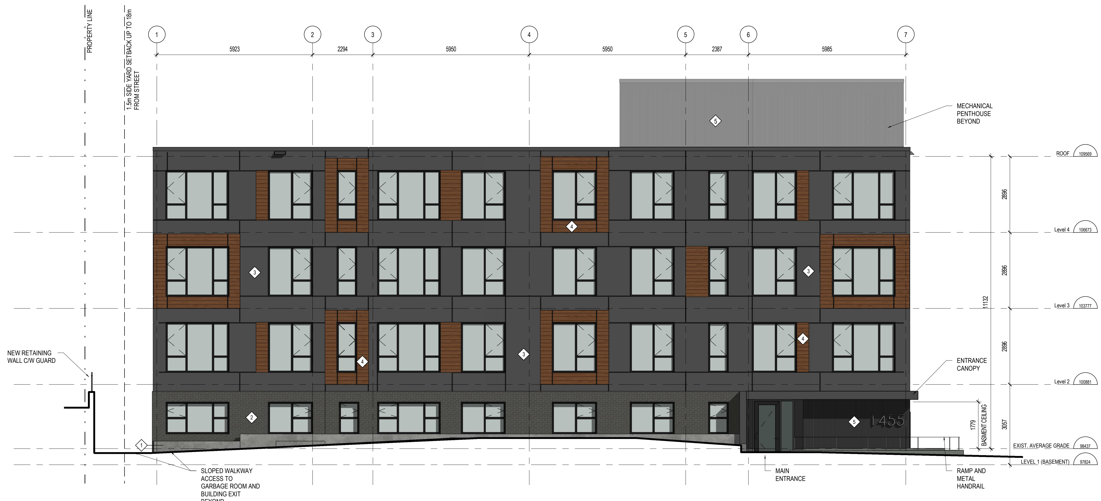
2 SOUTH ELEVATION ÉCHELLE / SCALE: 1:75
