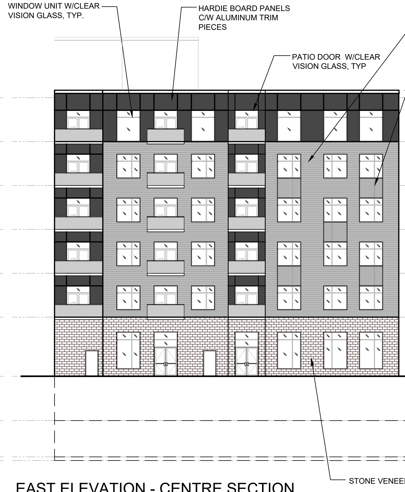
EAST ELEVATION - CENTRE SECTION SCALE: 1/16" = 1'-0"
