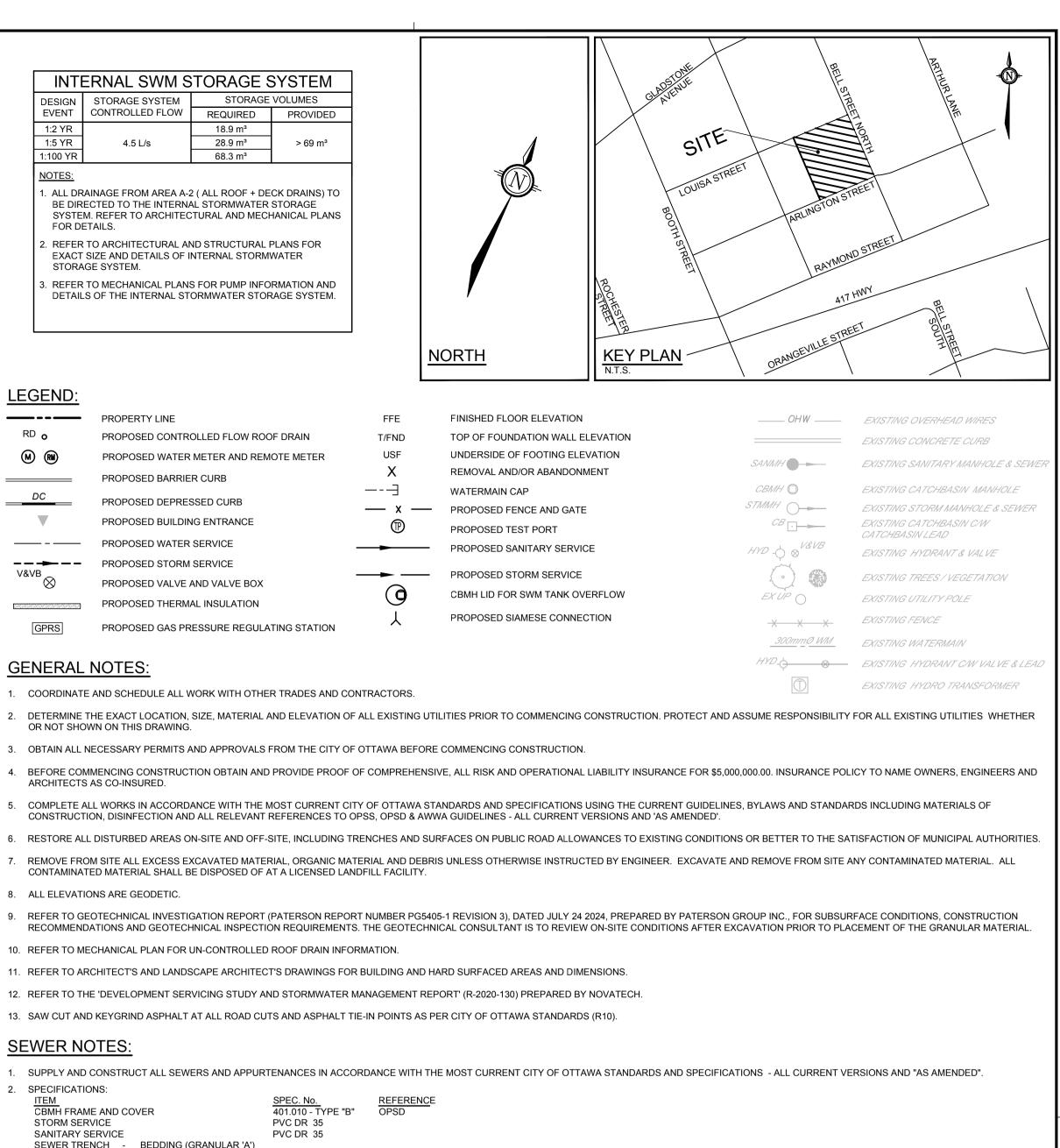
3. THE SANITARY SERVICE LATERAL SHALL BE EQUIPPED WITH A BACKFLOW PREVENTER WITHIN THE BUILDING FOOTPRINT AS PER CITY OF OTTAWA STANDARD DETAILS S14.1 OR S14.2. REFER TO MECHANICAL PLANS FOR 4. THE STORM SERVICE LATERAL SHALL BE EQUIPPED WITH A BACKFLOW PREVENTER WITHIN THE BUILDING FOOTPRINT AS PER CITY OF OTTAWA STANDARD DETAILS S14. REFER TO MECHANICAL PLANS FOR DETAILS.
