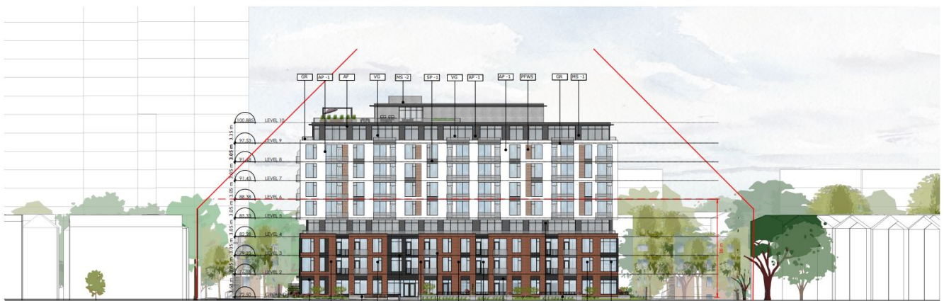
Figure 10: Angular Plane to the north and south of proposed building
