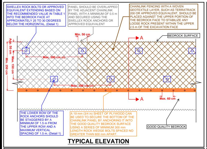
THE NUMBER OF ROWS AND LENGTH OF THE ROCK ANCHORS MAY BE CHANGED UPON EXPOSING THE BEDROCK SURFACE AND REVEALING THE BEDROCK CONDITIONS.
