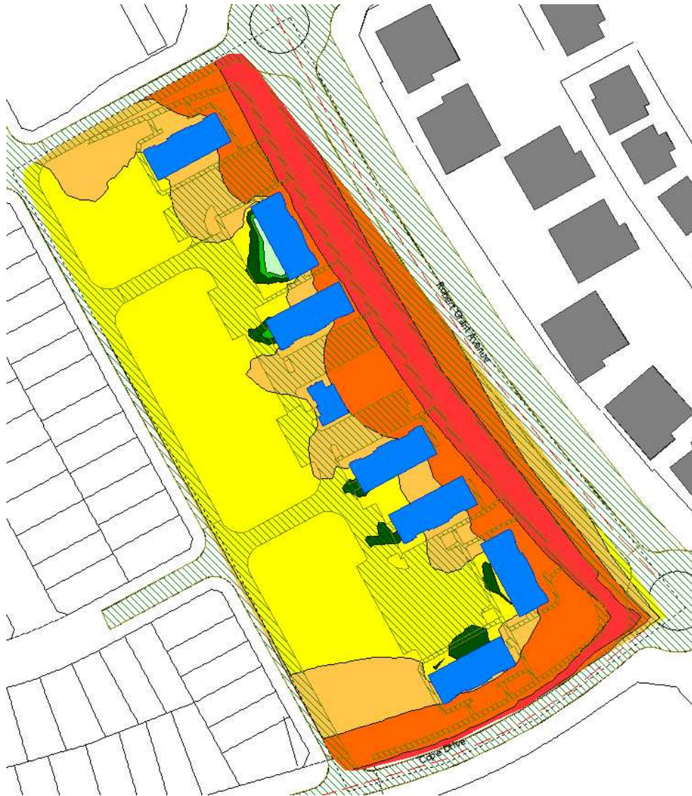
FIGURE 8: NIGHTTIME TRAFFIC NOISE CONTOURS (4.5 M ABOVE GRADE)
