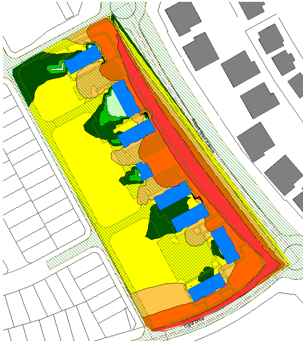
FIGURE 10: NIGHTTIME TRAFFIC NOISE CONTOURS WITH NOISE BARRIERS (1.5 M ABOVE GRADE)
