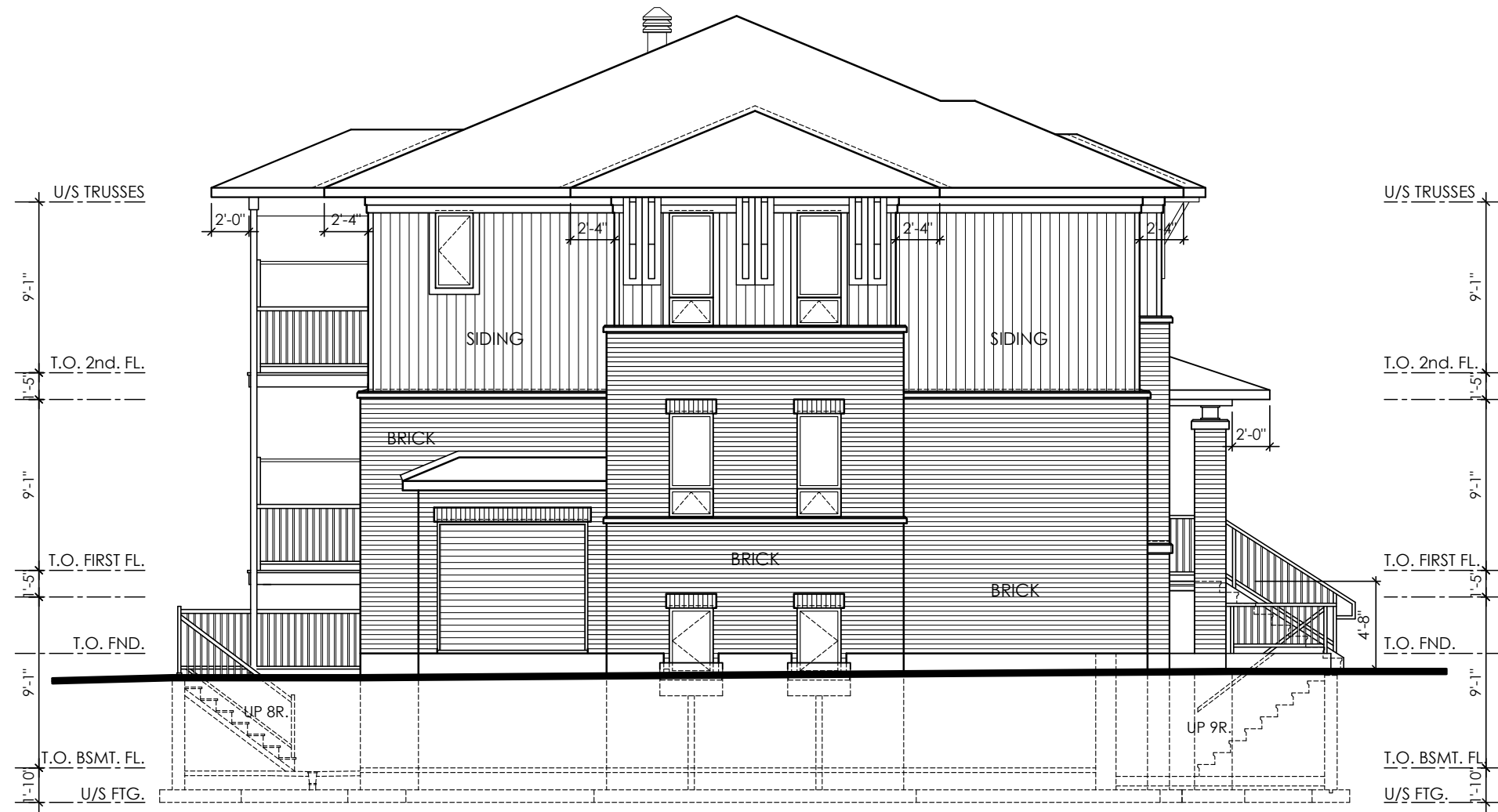
END UNIT UNIT 'A' UNIT 'B' UNIT 'C' END UNIT, STREET SIDE ELEVATION
