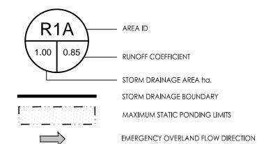
EXISTING EMERGENCY OVERLAND FLOW DIRECTION PROPOSED STORM SEWER PROPOSED CATCHBASIN PROPOSED WATTS AREA DRAIN OR EQUIVALENT
