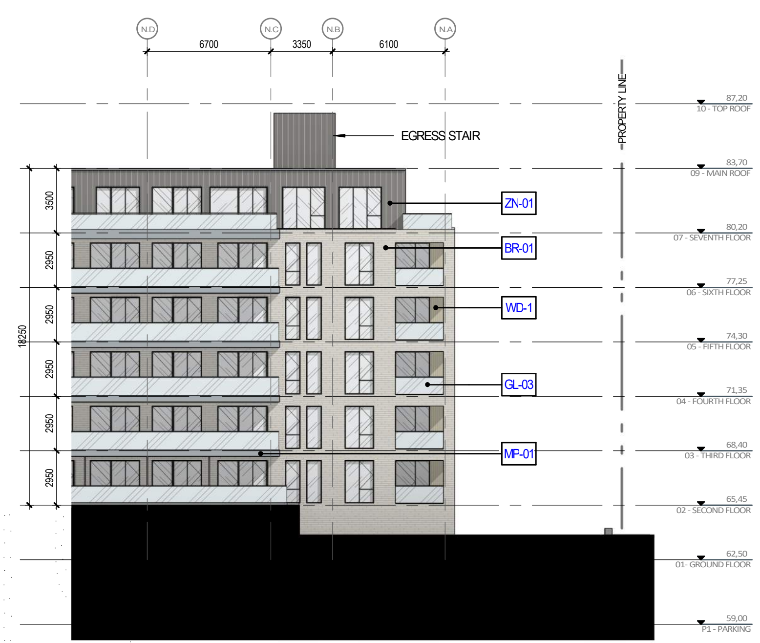
NORTH BUILDING NORTH ELEVATION 2 3 1:200 A.401
