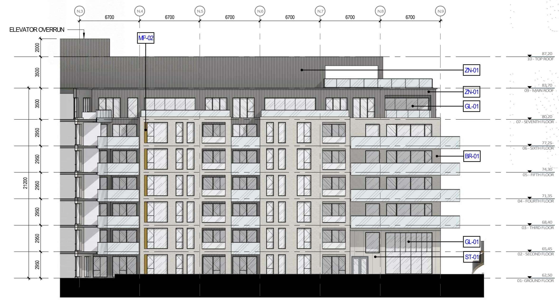
NORTH BUILDING - WEST ELEVATION 1 1 1:200 A.402
