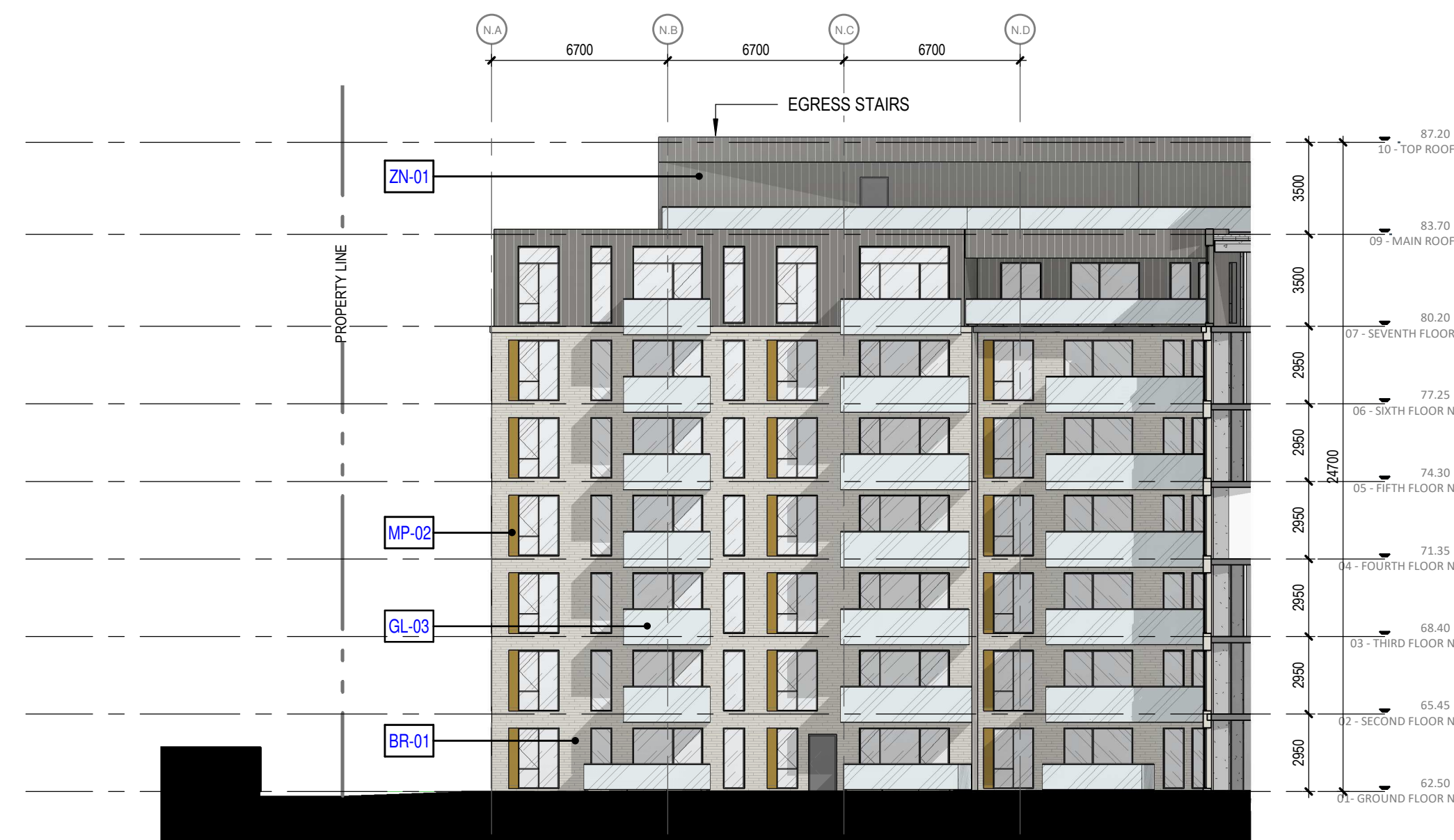
NORTH BUILDING - SOUTH ELEVATION 2 1 : 200
