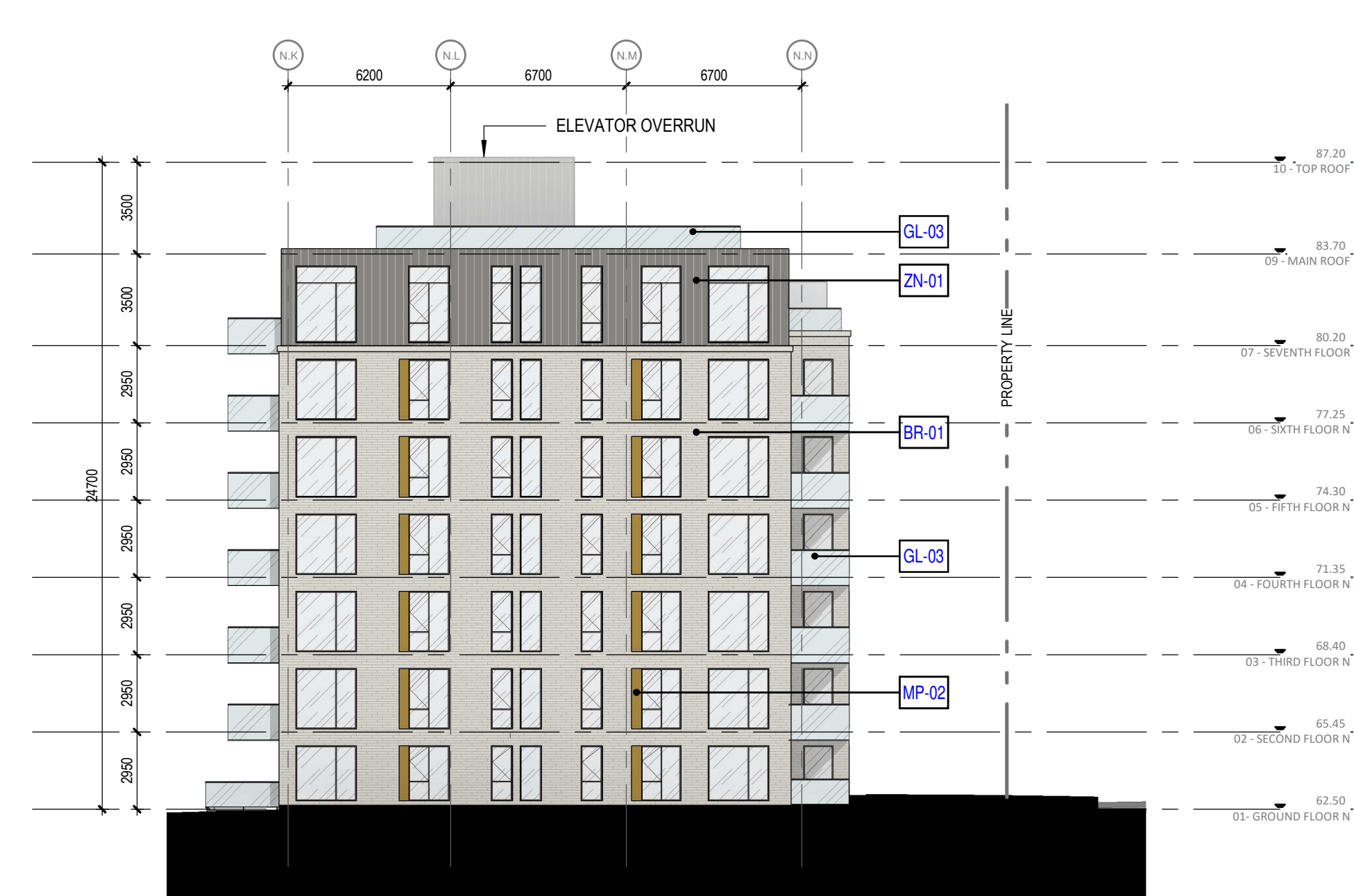
NORTH BUILDING - SOUTH ELEVATION 1 1 : 200
