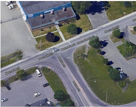
Figure 4 Unsignalized, with all-way stop-control
