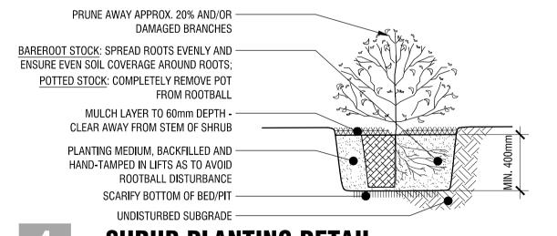
SEE PLANT LIST FOR SPACING MULCH LAYER TO 60mm DEPTH - CLEAR AWAY FROM BASE OF PLANT PLANTING MEDIUM, BACK FILLED AND HAND-TAMPED IN LIFTS AS TO AVOID ROOTBALL DISTURBANCE UNDISTURBED SUB GRADE
