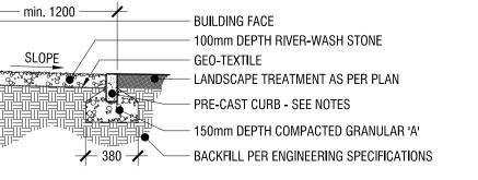
RIVER-WASH STONE TO BE COLOURED, SIZED 40-65mm Ø. PRE-CAST CURB TO BE INTERLOCKING "Universal Curb" AS MANUFACTURED BY Permacon OR APPROVED EQUIVALENT. USE CORNER UNITS AT ALL 90° CORNERS. PRE-CAST CURB MAY BE SUBSTITUTED WITH 6x6 PRESSURE-TREATED TIMBER OR COMMERCIAL GRADE ALUMINUM EDGER UPON APPROVAL.
