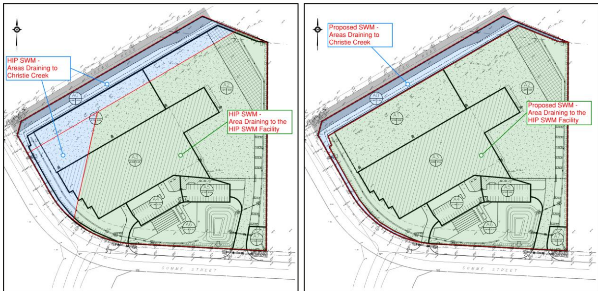
Figure 4-1 SWM Drainage Area from HIP SWM (left), and from Proposed SWM (right)
