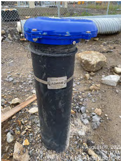
Photo 5 - Observation well (ID A295342) used during pumping test for monitoring of potential interference effects.
