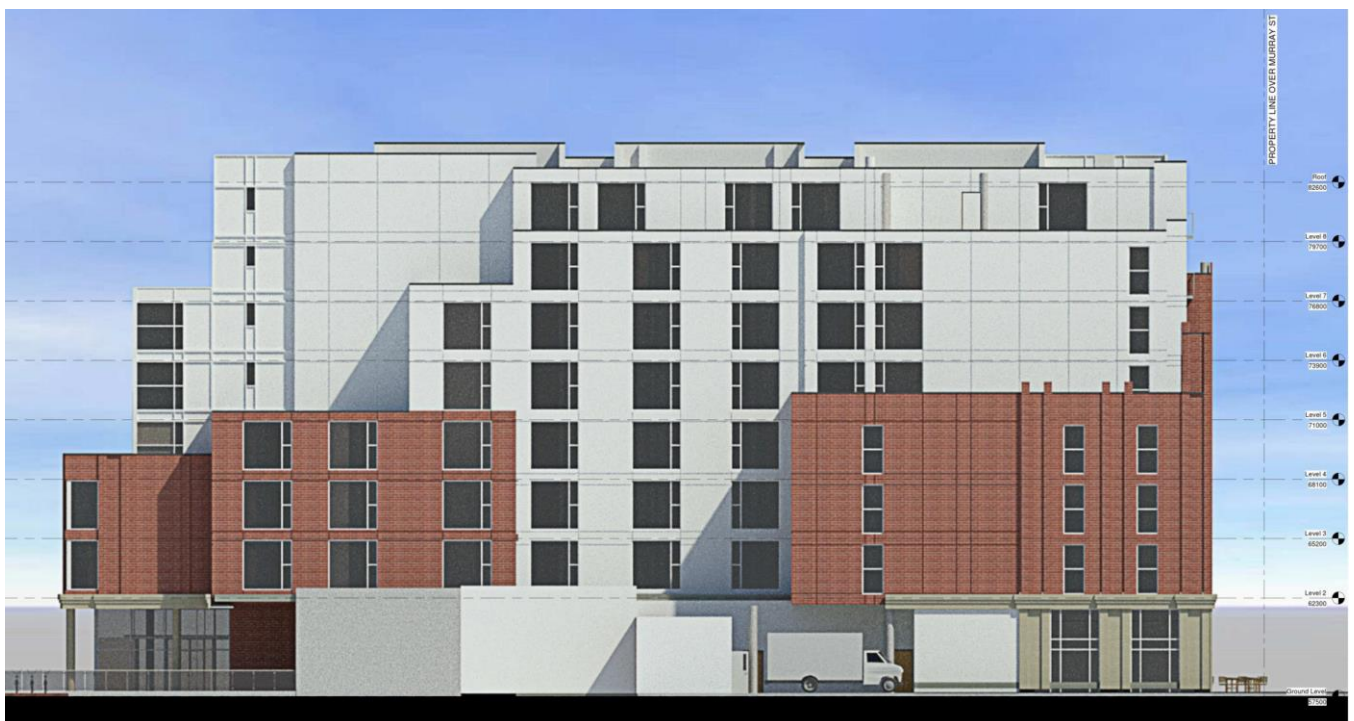
Figure 12: The East Elevation needs to be cleaned up in line with the other elevations. The brick should be carried around the building. The neighbouring buildings are low and east west views tend to be the most prominent. Source: Woodman Architect & Associates. 2021
