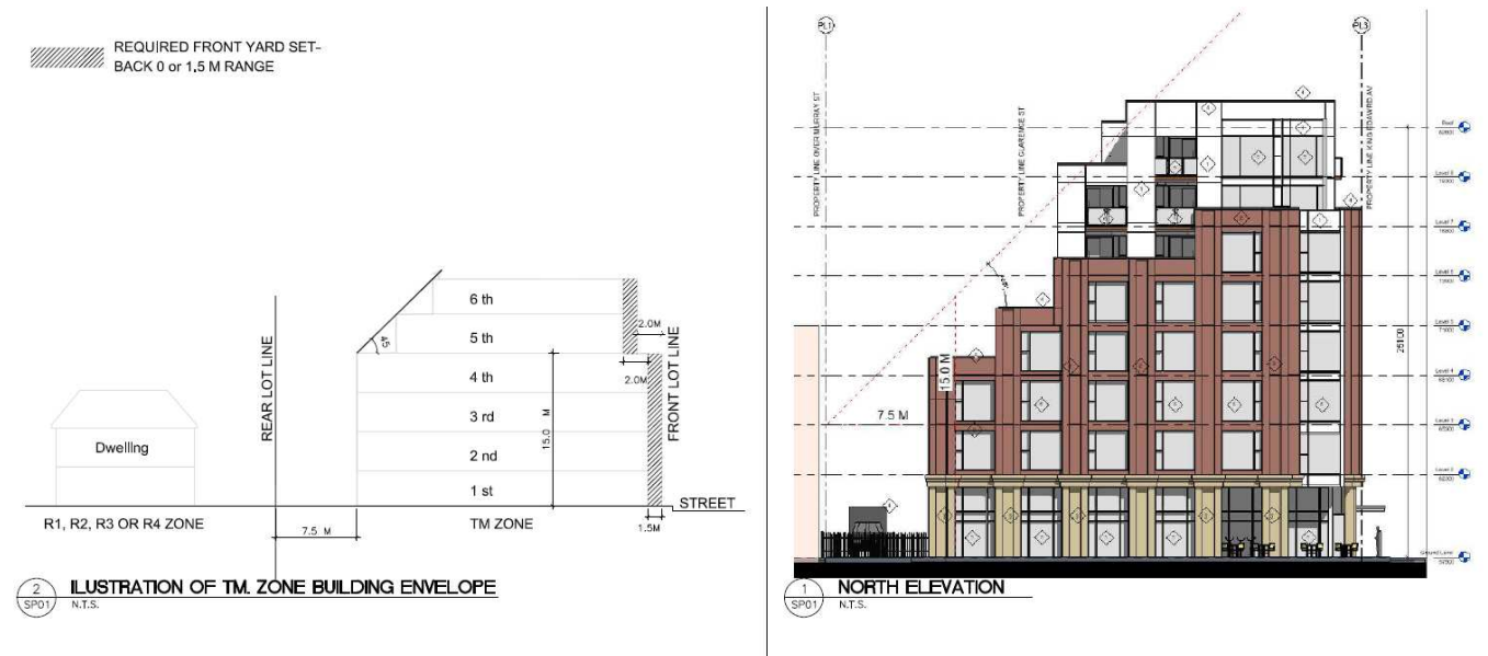
Figure 10: Illustration of the TM building envelope with the 45-degree angle respecting the adjacent property.
