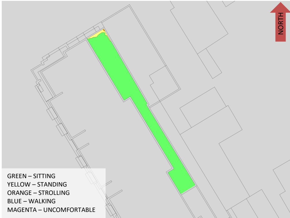
FIGURE 4A: SPRING – WIND COMFORT, LEVEL 7 AMENITY TERRACE
