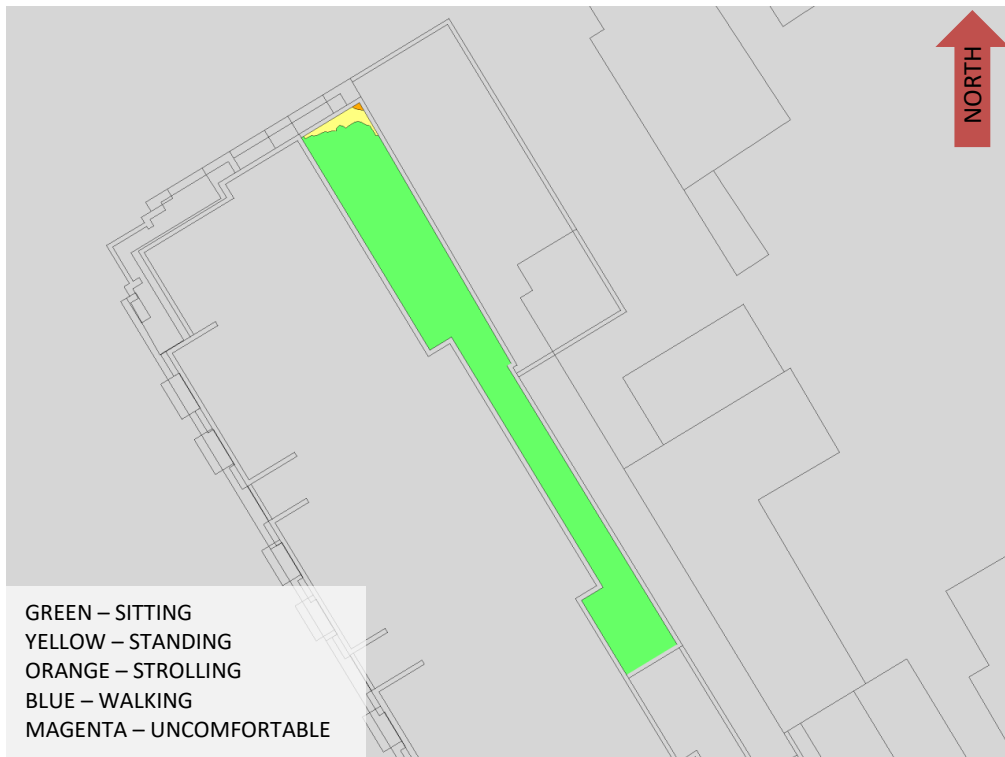
FIGURE 4D: WINTER – WIND COMFORT, LEVEL 7 AMENITY TERRACE
