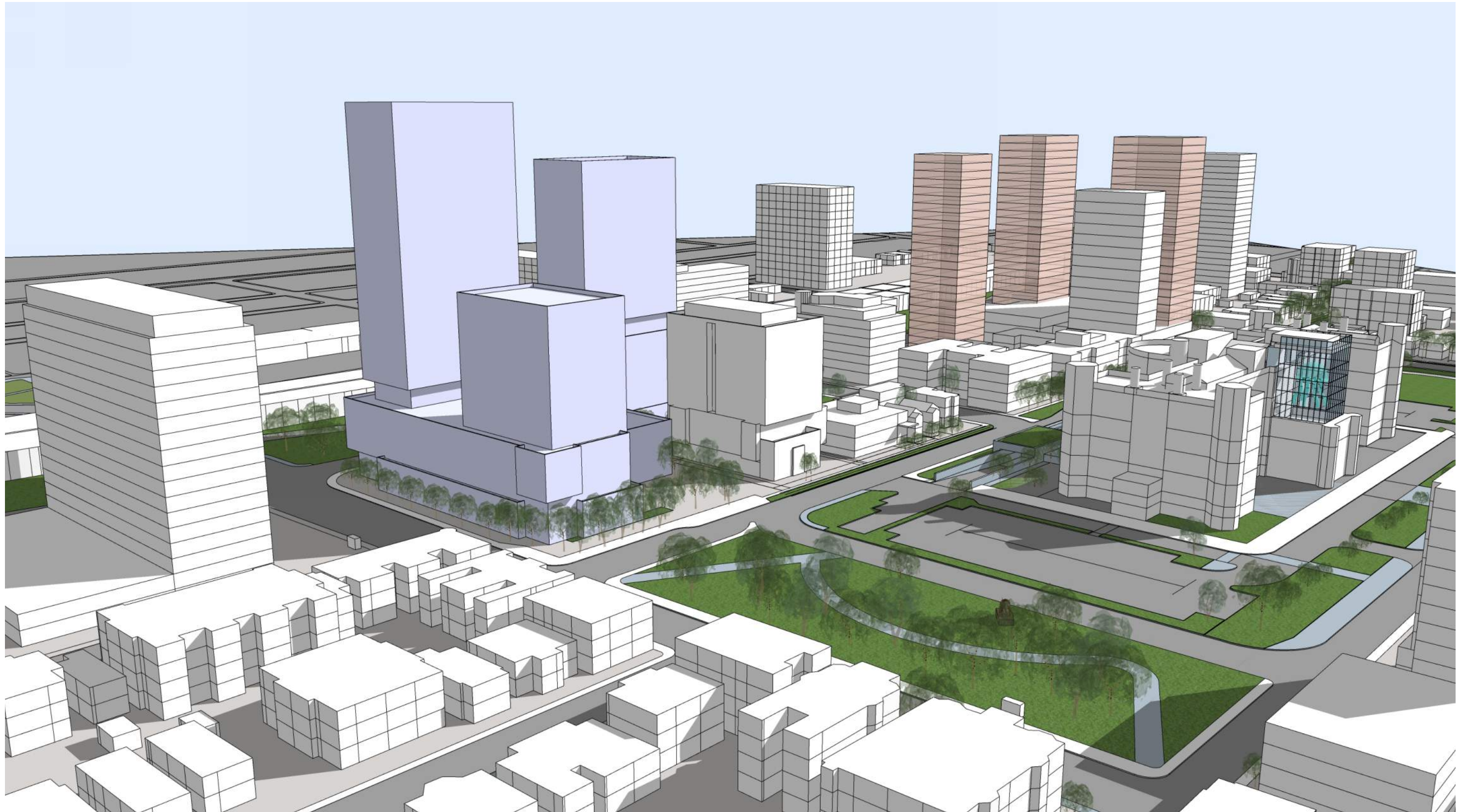
The Massing Model demonstrates the compatibility of the newly developed proposed 12-storey project with the Museum of Nature, and the projected context study of Argyle, Elgin and Catherine streets (shown in blue). The transition in height and scale from Catherine Street (30 storeys) to the 12-storey proposed 100 Argyle is commensurate with both the goal of the Secondary Plan and the CDP which seeks to have a mediating scale of buildings encircling the Museum of Nature and the park area around it.
