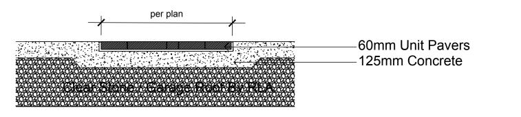
UNIT PAVING WITHIN CONCRETE
