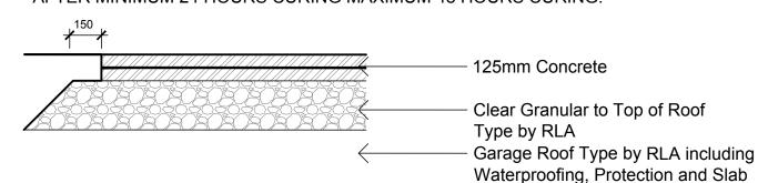
CONCRETE PAVING TYPE 1 & TYPE 2
