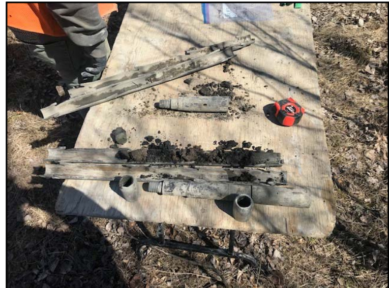
Photo 4: Spoon BH1 S2 - Asphalt Layer 0.8 to 0.9 m Depth - April 7-2021
