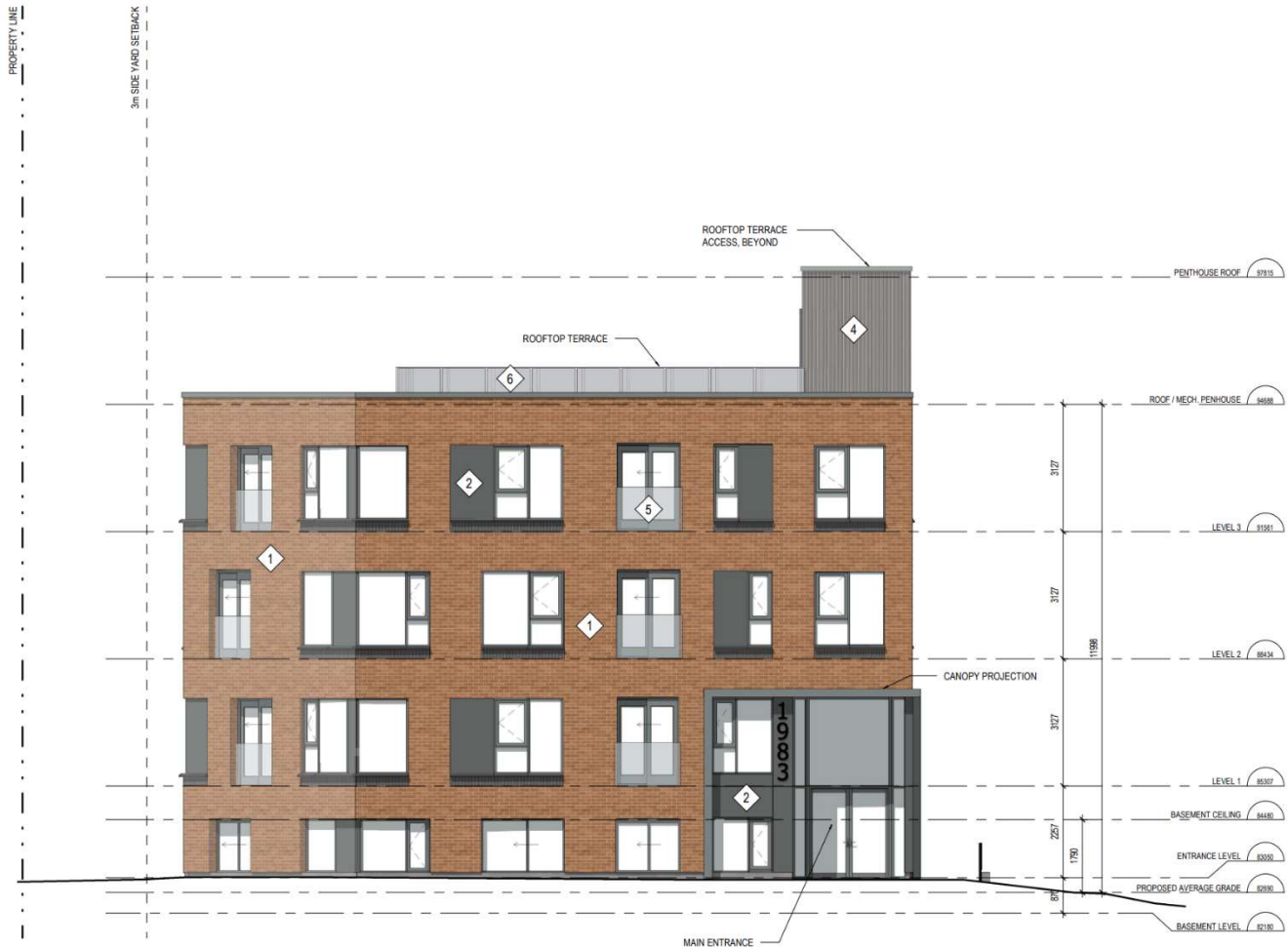
Exhibit I-1: South Elevation (facing Carling Avenue)
