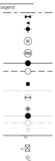
PROPOSED WATERMAIN PROPOSED VALVE AND VALVE BOX PROPOSED REDUCER PROPOSED FIRE HYDRANT
