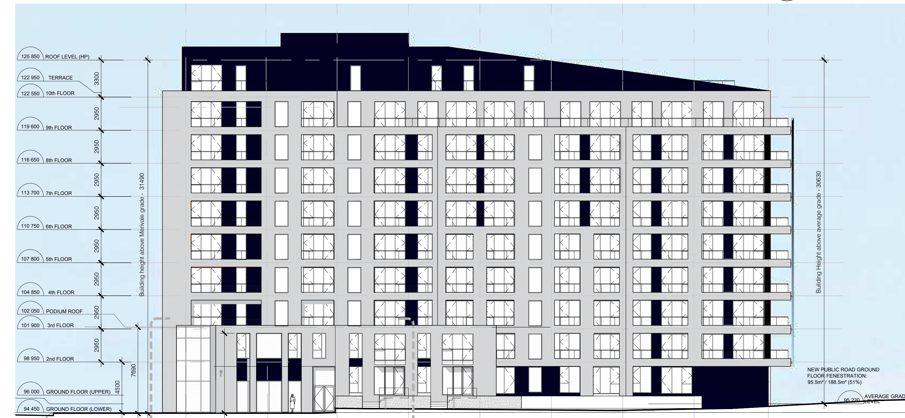
ELEVATION EAST - NEW PUBLIC ROAD PHASE 1 1:200 A300
