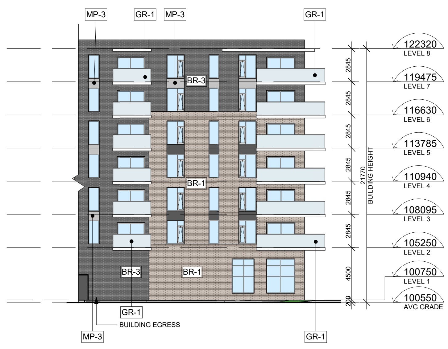
3 WEST ELEVATION - WEST BUILDING 1 : 200
