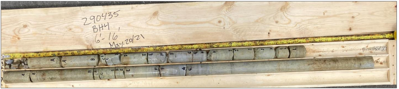
Photo 1 – Borehole BH4, Rock Core (Runs 1 and 2)
