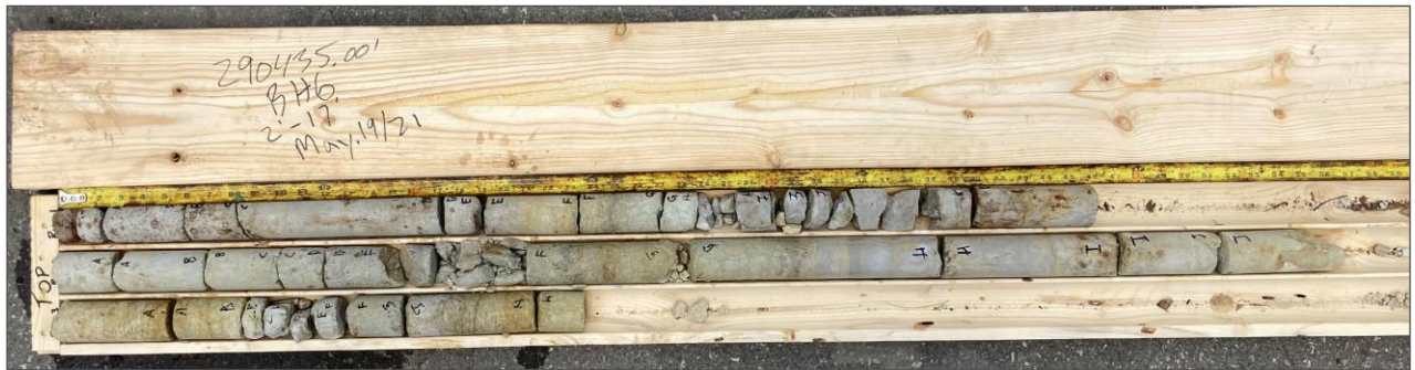
Photo 2 – Borehole BH6, Rock Core (Runs 1 to 3)
