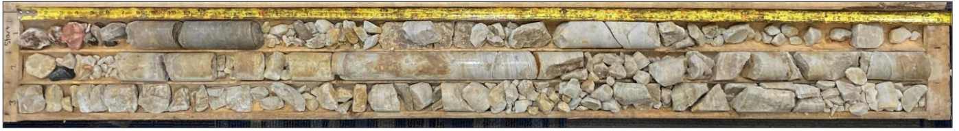
Photo 4 – Bedrock Probe RP4, Rock Core (Runs 1 to 3)
