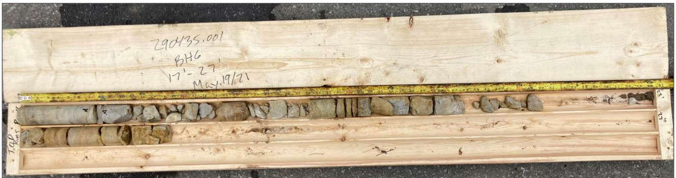
Photo 3 – Borehole BH6, Rock Core (Runs 4 and 5)
