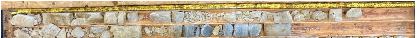
Photo 6 – Bedrock Probe RP9, Rock Core (Runs 4 and 5)
