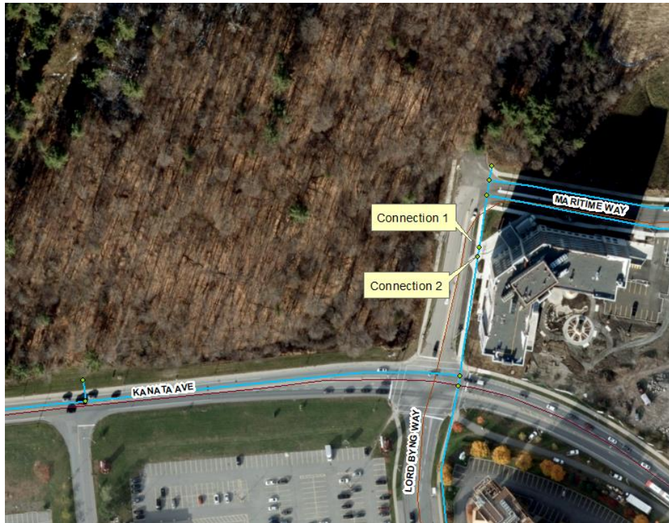
Figure 1: Service connection locations for the water distribution system (City of Ottawa)
