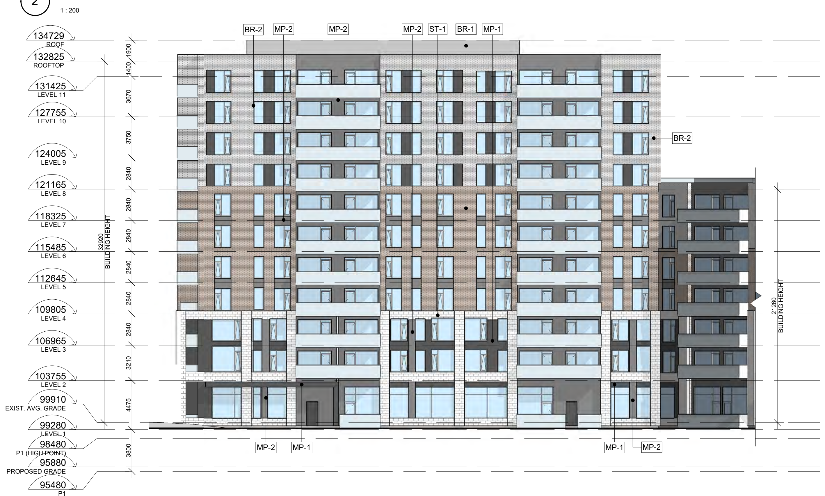
3 NORTH ELEVATION - EAST BUILDING 1:200
