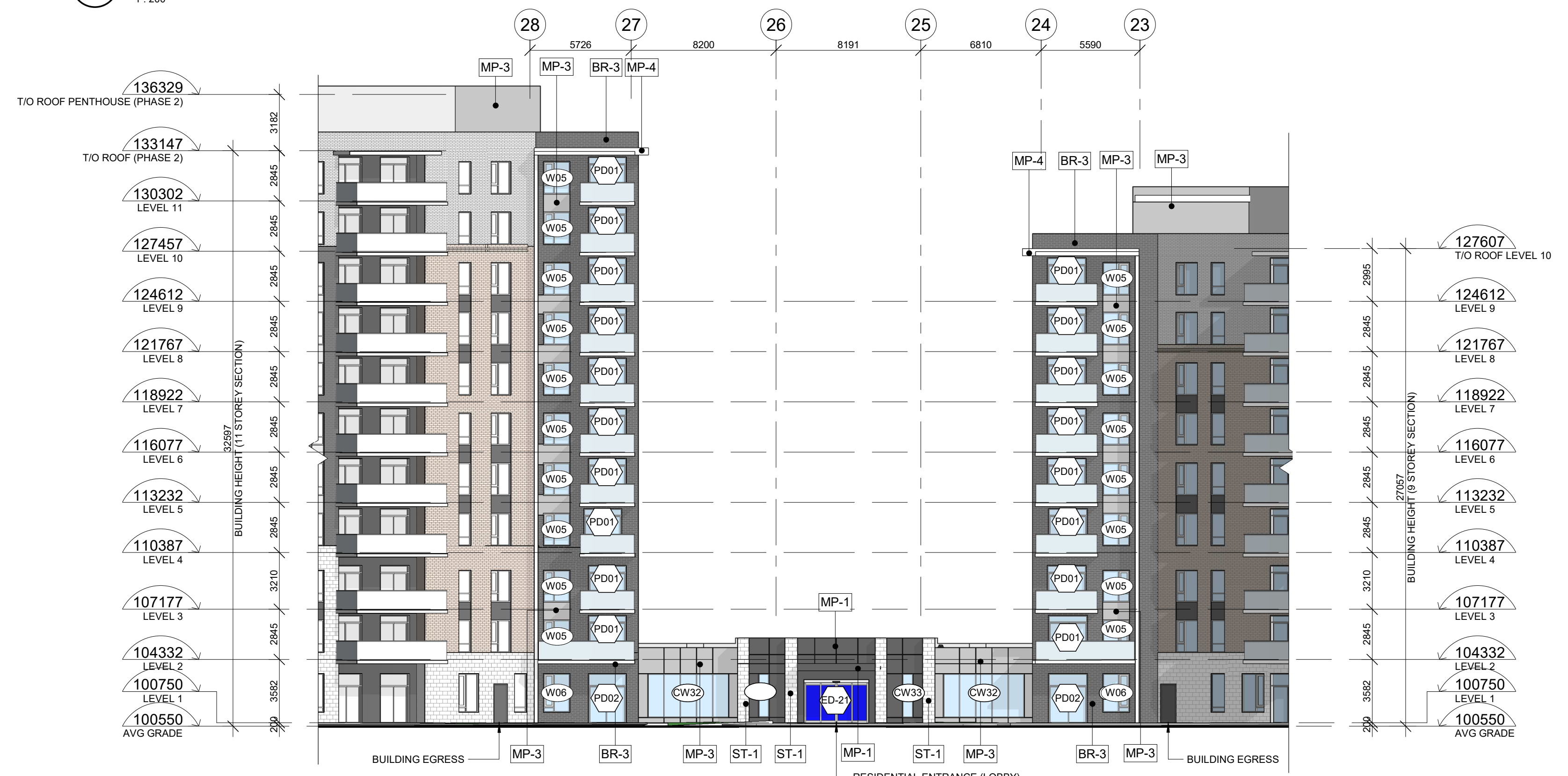
3 NORTH ELEVATION - CENTRE BUILDING 1 : 200
