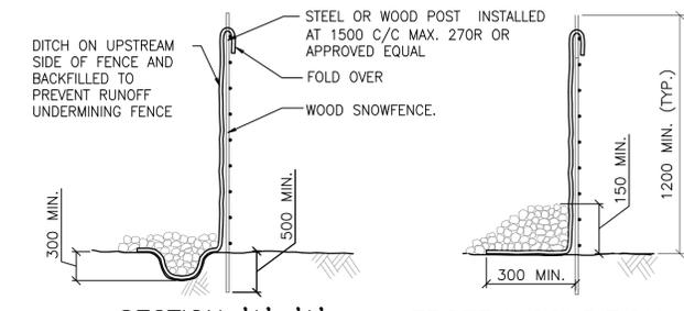
**3 TYP. CATCHBASIN SEDIMENT PROTECTION DETAIL**
