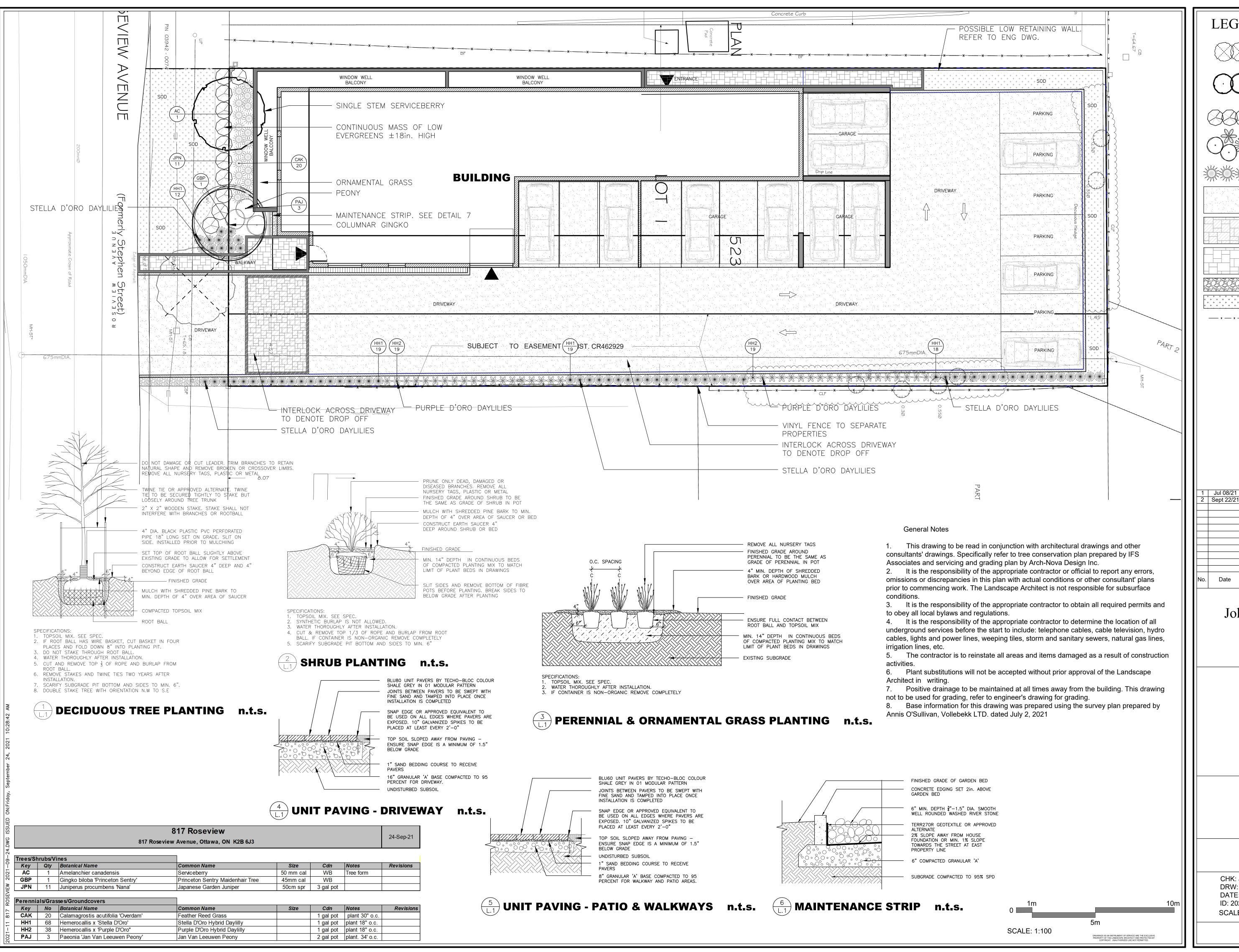
**LEGEND** EXISTING DECIDUOUS TREE TO BE REMOVED PROPOSED DECIDUOUS TREE PROPOSED SHRUBS PROPOSED PERENNIALS PROPOSED GRASSES ASPHALT HEAVY DUTY UNIT PAVING. SEE DETAIL 5 ON L.1 LIGHT DUTY UNIT PAVING. SEE DETAIL 6 ON L.1 RIVER ROCK ON BLACK FILTER CLOTH — × — × — EXISTING FENCE
