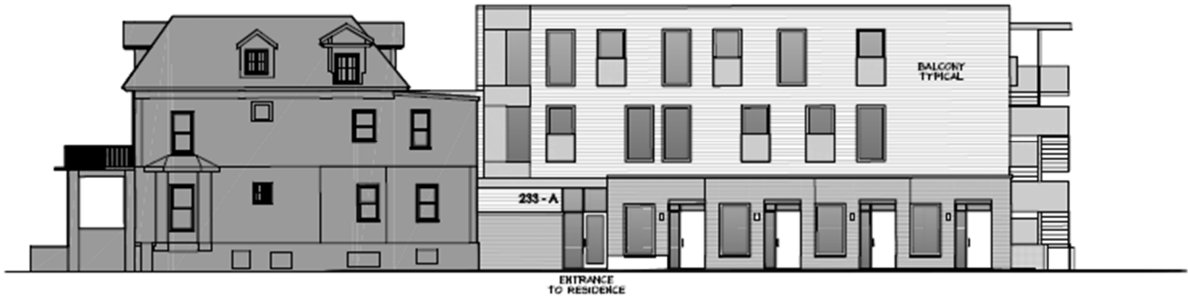
Figure 9: East Elevation of the proposed addition
