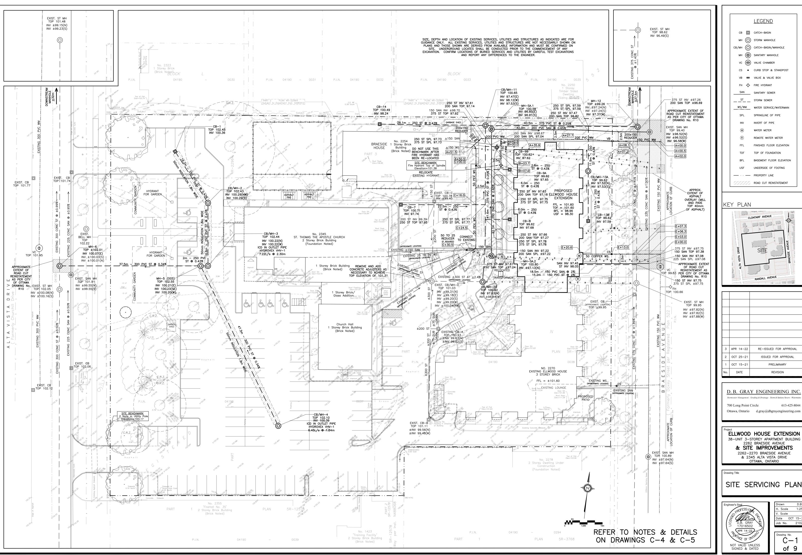
**LEGEND** CB 🔲 CATCH-BASIN MH (O) STORM MANHOLE CB/MH (C) CATCH-BASIN/MANHOLE MH ( ) SANITARY MANHOLE VC ( VALVE CHAMBER CS • CURB STOP & STANDPOST VB 💌 VALVE & VALVE BOX FH -O- FIRE HYDRANT SANITARY SEWER \_\_\_Sr\_\_\_ STORM SEWER WS/WM WATER SERVICE/WATERMAIN SPRINGLINE OF PIPE INVERT OF PIPE WATER METER REMOTE WATER METER FINISHED FLOOR ELEVATION TOP OF FOUNDATION BASEMENT FLOOR ELEVATION UNDERSIDE OF FOOTING
